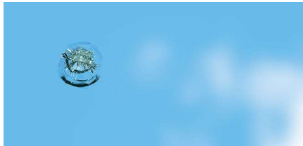
Cracked glass less than 1/2" in diameter
