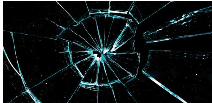
Cracked glass equal to or more than 1/2" in diameter or spidered cracks
