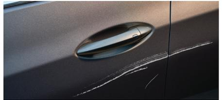
1 dent over 4” or 1 scratch equal to or over 6” per panel
